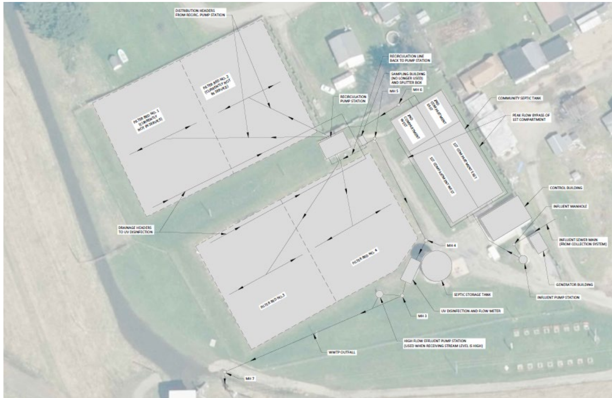
EXISTING WWTF SITE PLAN
