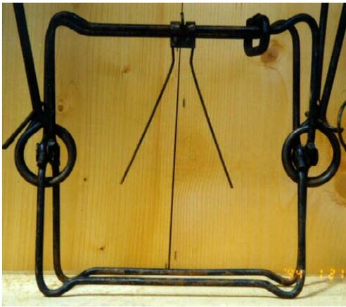
**FIGURE 5.** #330 with a Standard V Trigger configuration.
