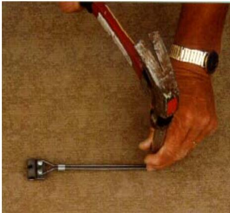
**STEP 3.** Slide the two ferrules on the trigger wires and crimp using the cold chisel/screw driver and hammer. Crimp the splicing sleeves at the top and bottom of the now parallel wires.
