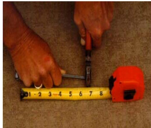
**STEP 2.** Assemble the bolt on replacement trigger. Pinch the wires together and measure down 6 1/2" from the bottom of the trigger clamp and cut off the wires at this length.
