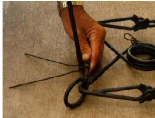
**STEP 1.** Remove the existing trigger using the cold chisel or screw driver and hammer. Most stock triggers are attached by rivets. These you will need to cut or pry apart in order to remove the old trigger.
