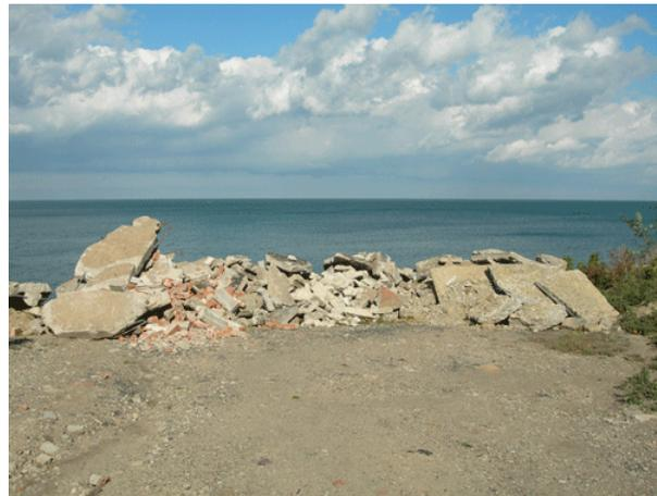
*The above photo shows typical concrete rubble of greatly varying size. The larger slabs may not be suitable as filter layer material.*
