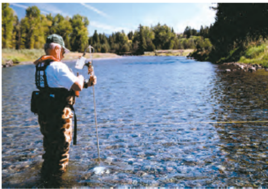
Figure 17. Wading measurement using a top-setting rod.
