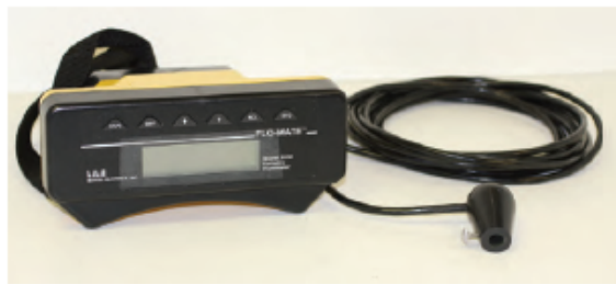
Figure 38. Marsh-McBirney Model 2000 electromagnetic flowmeter and display meter.
