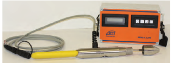
Figure 39. Ott electromagnetic current meter.
