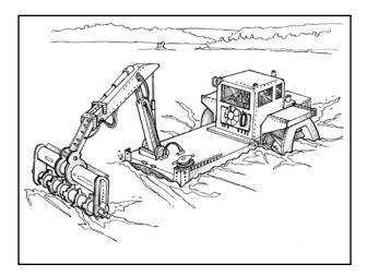
Fig. 6–6. Rotovating equipment uses large cutters to remove aquatic plants and their roots from lake sediments. (CREDIT: CHRIS COOLEY)
