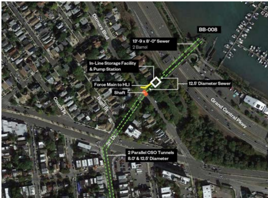
Figure 8-19. Layout of Alternative 9-3 – Outfall Storage for BB-008
