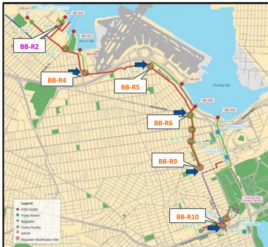
Figure 4-2. Flushing Bay High Level Interceptor Regulator Improvements
