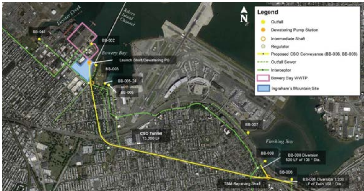
Figure 8-23. Conceptual Layout of Alternatives 9-7a, 9-8a and 9-9a – Tunnel Storage for 25%, 50% and 75% CSO Control at the Ingraham's Mountain Site
