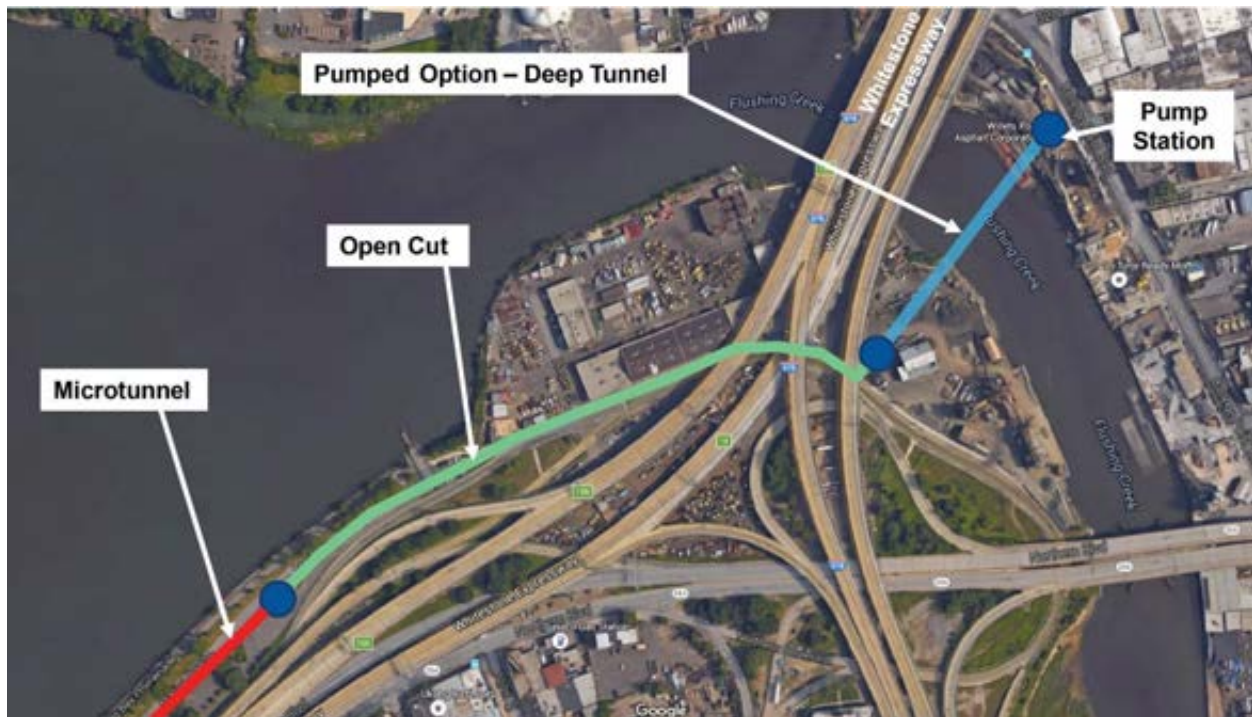
Figure 8-12. Layout of Alternative 7-2b – Extension of the BB HLI Consolidation Conduit to Address from Flushing Creek Outfall TI-011
