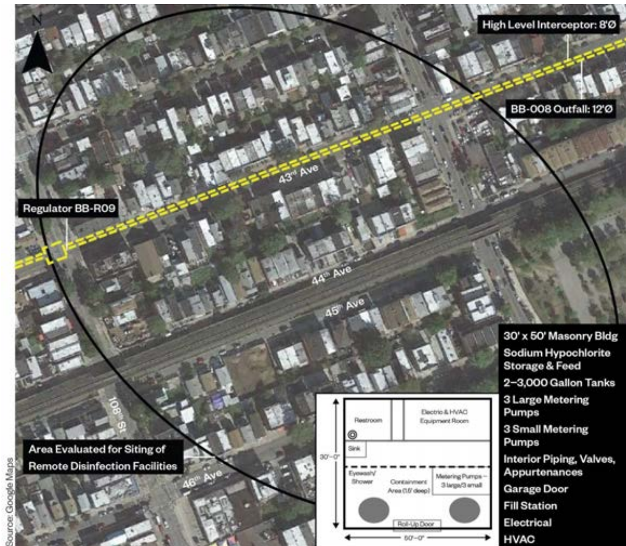
Figure 8-14. Alternative 9-1 – Remote Disinfection Facility for Outfall BB-008
