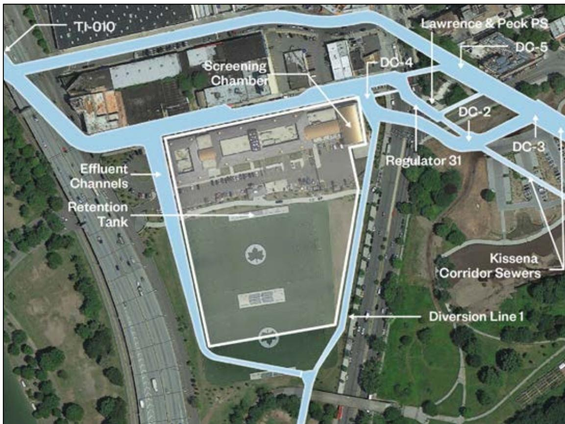
**Figure 1: Sewer Configuration Upstream of TI-010**
