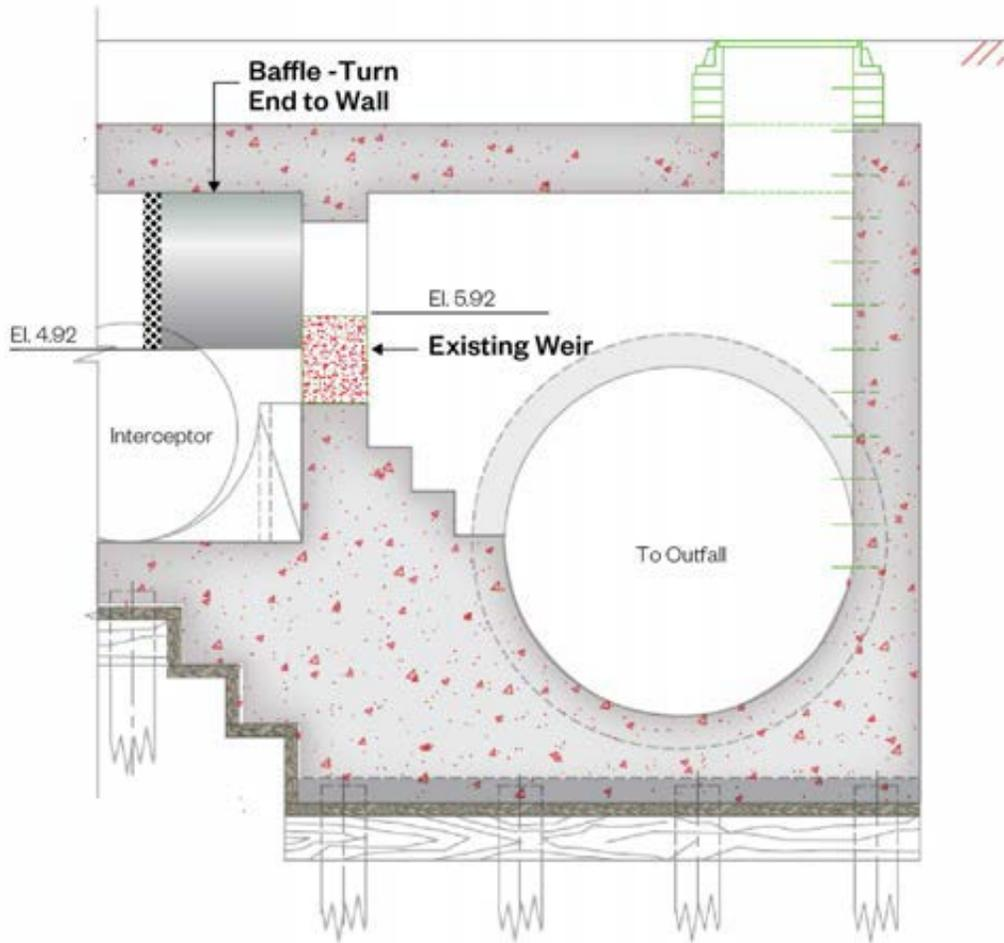
Figure 5: TI-R09 Baffle Concept – Existing Weir Configuration
