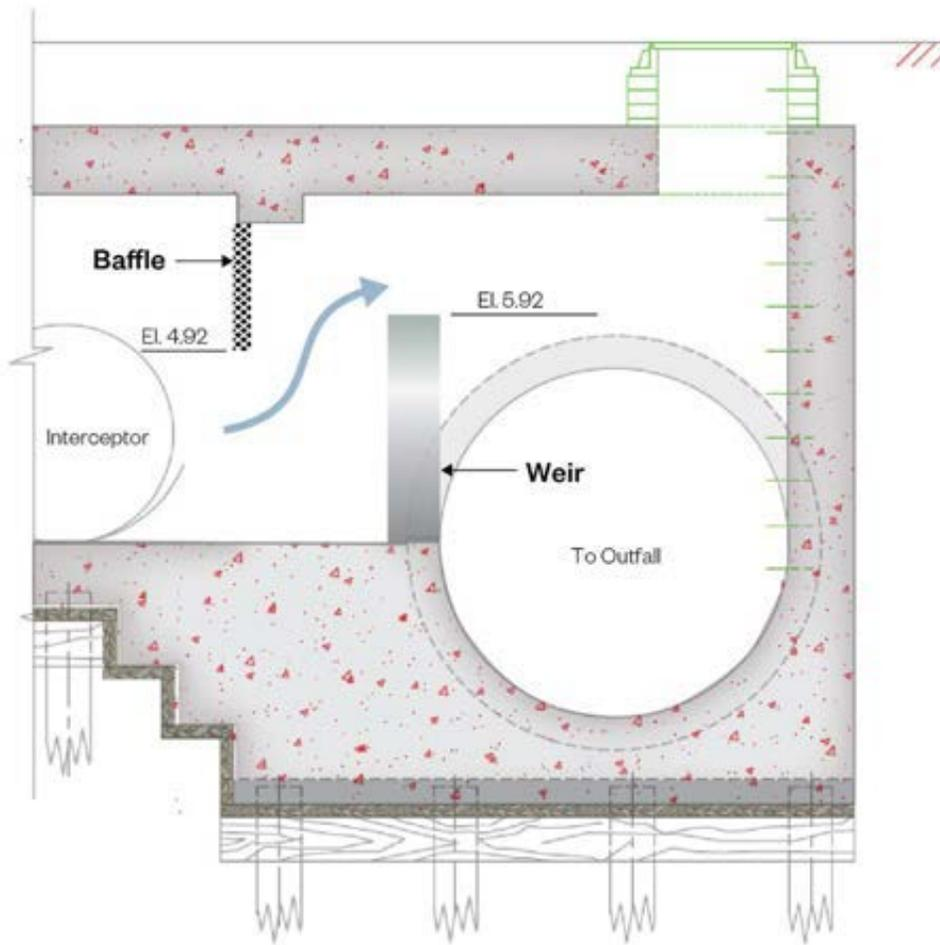
Figure 6: TI-R09 Baffle Concept – Revised Weir Configuration
