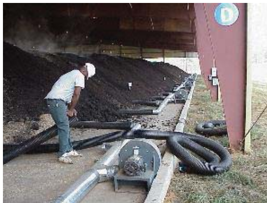
Figure A-14-3. Forced aeration systems, or aerated static piles, use blowers to provide oxygen into the compost pile instead of turning or moving the pile. Photo: Jason Governo, U. of Georgia
