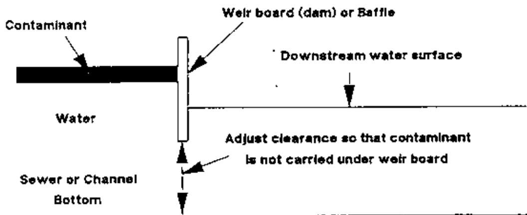
When current flow exceeds 3 ft/sec, contaminants can be trapped by creating a difference in upstream and downstream surface with a baffle or weir board.
