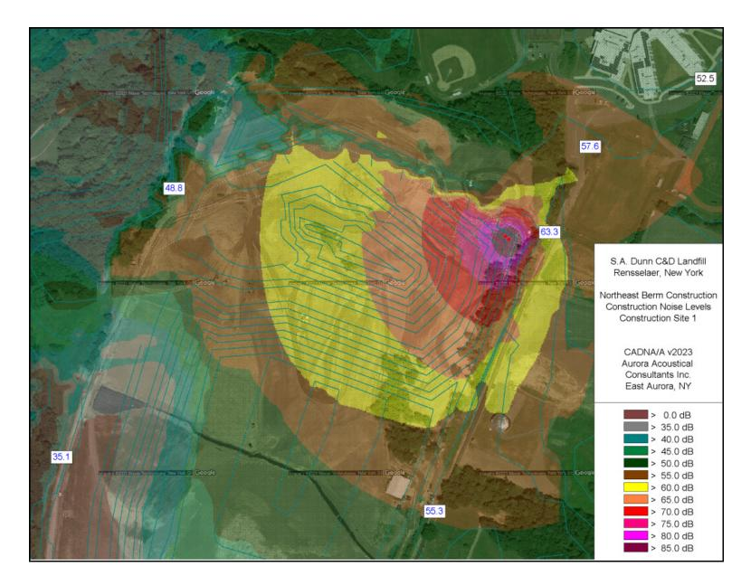
Figure 2 Modeled sound levels from planned berm construction operations at Construction Site 1
