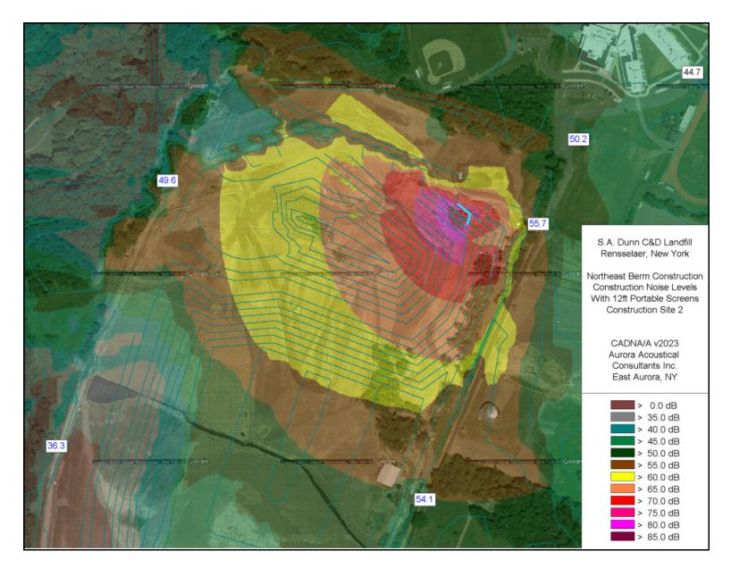
Figure 7 Modeled sound levels from planned berm construction operations at Construction Site 2, mitigated
