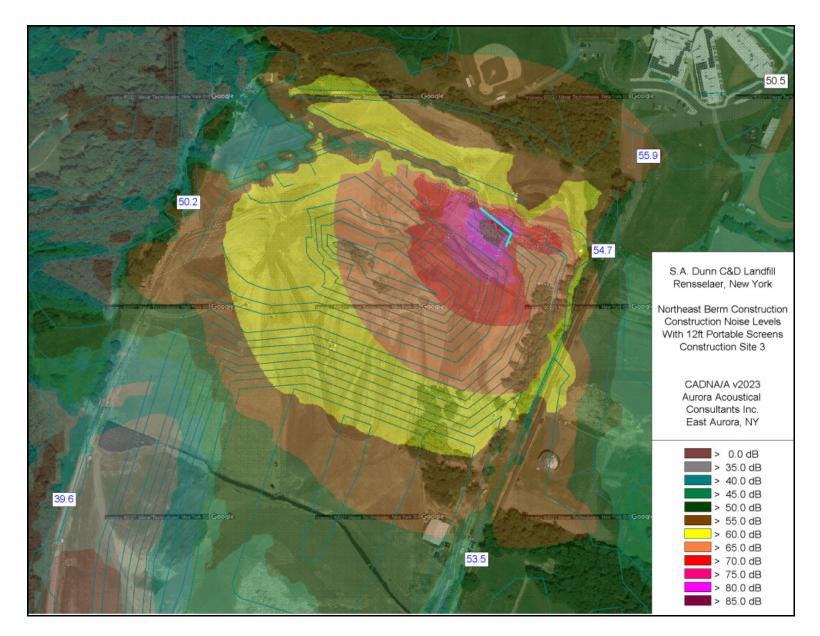
Figure 8 Modeled sound levels from planned berm construction operations at Construction Site 3, mitigated
