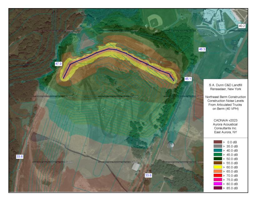
Figure 10 Modeled sound levels from pass-bys of articulated trucks on planned northeast MSE berm
