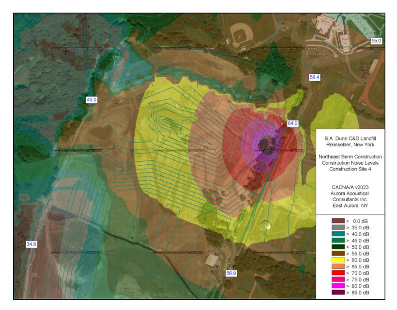
Figure 5 Modeled sound levels from planned berm construction operations at Construction Site 4
