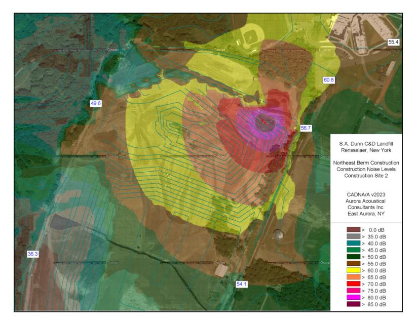
Figure 3 Modeled sound levels from planned berm construction operations at Construction Site 2
