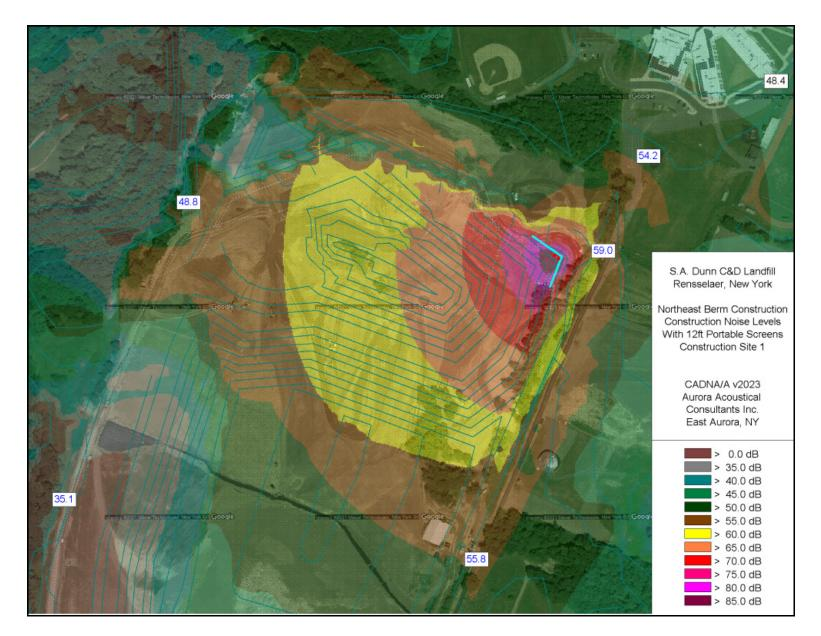
Figure 6 Modeled sound levels from planned berm construction operations at Construction Site 1, mitigated
