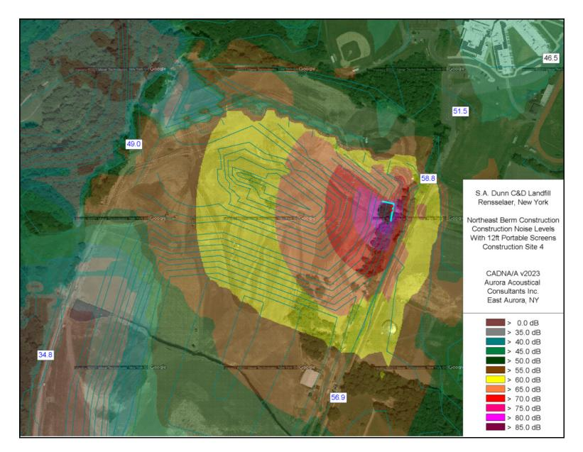
Figure 9 Modeled sound levels from planned berm construction operations at Construction Site 4, mitigated
