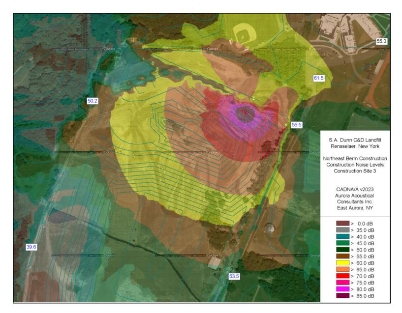
Figure 4 Modeled sound levels from planned berm construction operations at Construction Site 3
