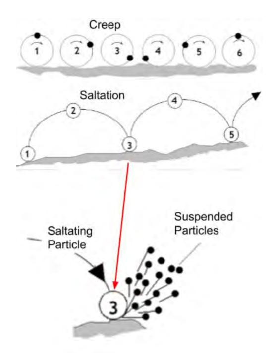
Figure 1. Illustration of the wind erosion process
