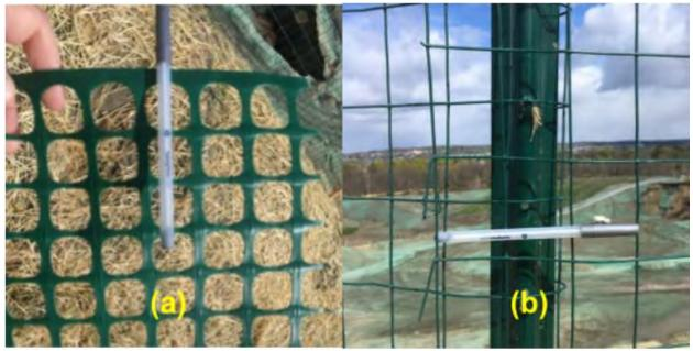
Figure 8. Plastic and welded wire fence materials
