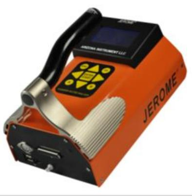
A handheld Jerome meter is used to detect low concentrations of hydrogen sulfide at levels that people usually begin to observe
