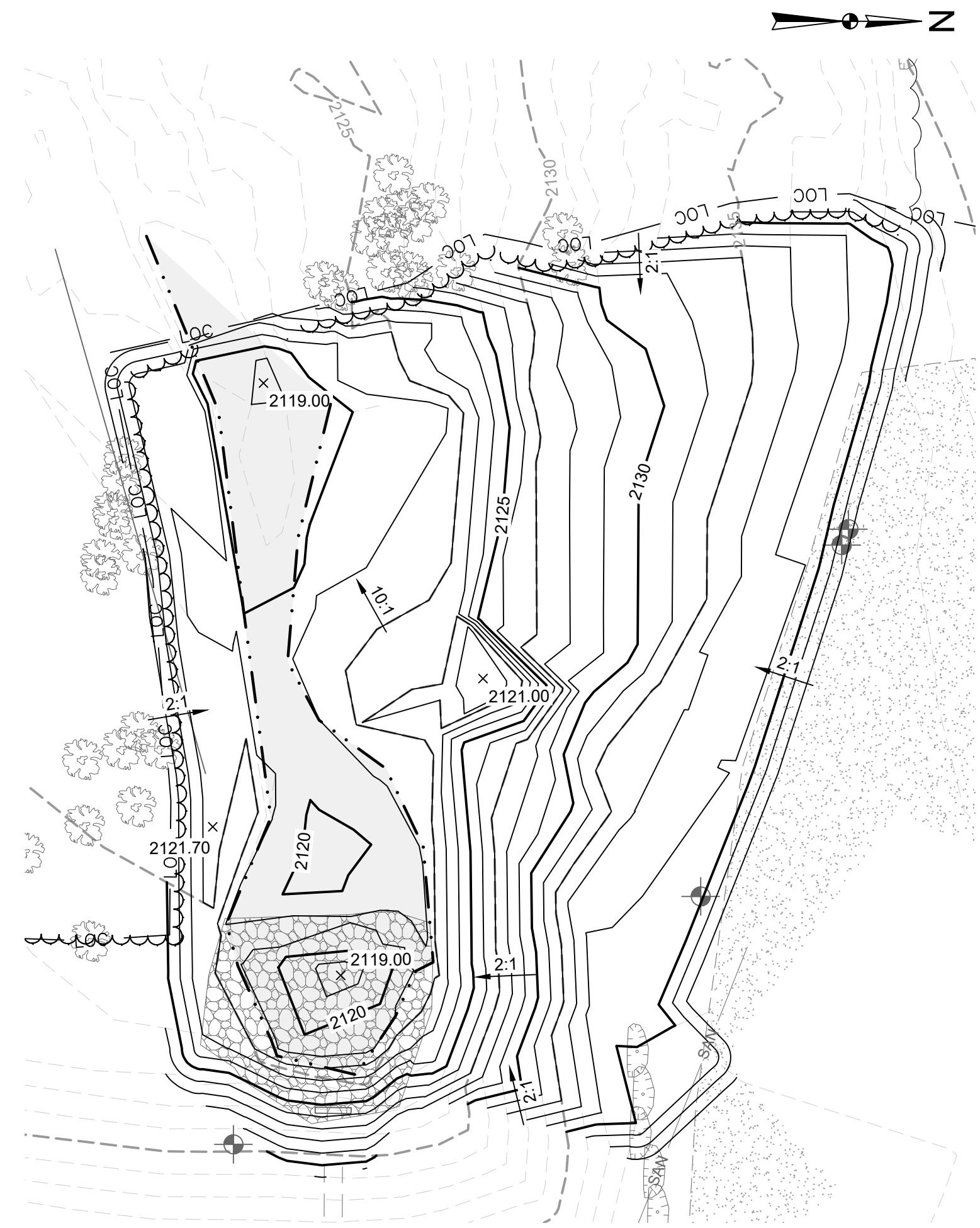
AUXILIARY SPILLWAY AND PLUNGE POOL EXCAVATION PLAN
