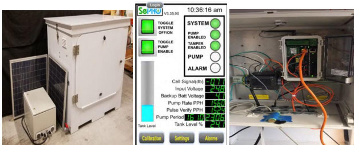
Figure 3: A fluridone injection unit (left), unit control dashboard (center), and cellular control device (right). SePRO
