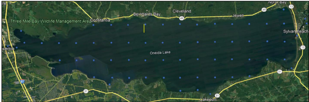
Figure 1. Approximate locations of the acoustic telemetry receiver array at 2km spacing in the lake and additional receivers in major tributaries. Actual locations will be determined after receiver range tests are conducted in summer 2023.
