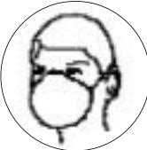
**Approved filtering facepieces (dust masks)** can be used for dust, mists, welding fumes, etc. They do not provide protection from gases or vapors. DO NOT USE FOR ASBESTOS OR LEAD; instead, select from the respirators below.
