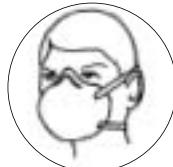
**Half-face respirators** can be used for protection against most vapors, acid gases, dust or welding fumes. Cartridges/filters must match contaminant(s) and be changed periodically.
