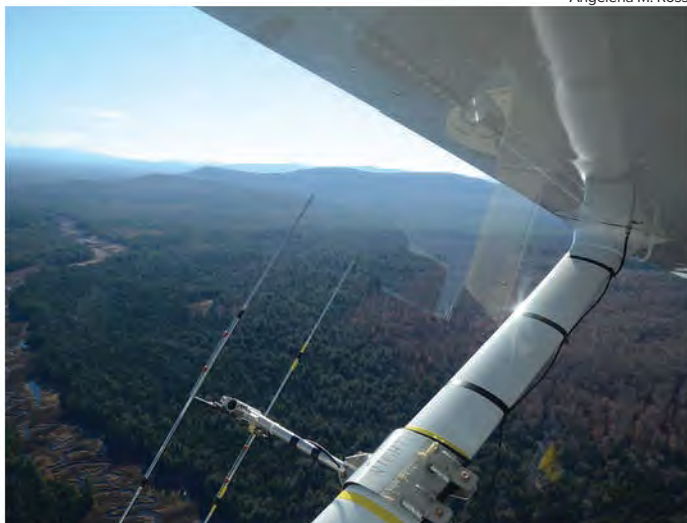
Radio telemetry allows biologists to track collared birds. Here, biologists fly over an area trying to pick up the radio signals emitted by the transmitters in the birds' collars.
