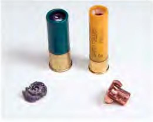
Shotgun slugs made of copper (right) fold nicely down into "petals" expanding the slug's surface area better than slugs made of lead (left).
