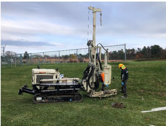
Drill rig collecting soil and groundwater samples at Algonquin Middle School
