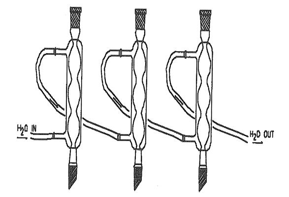
Figure 2: Allihn Condensers Connected in Series
