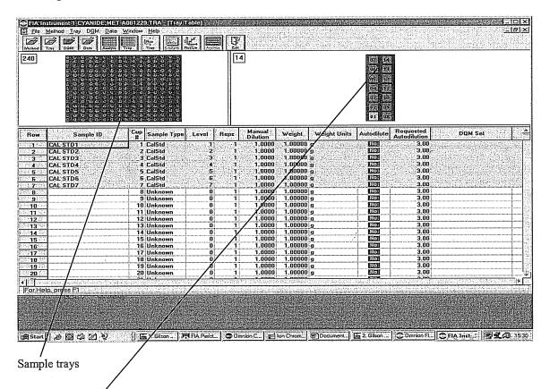
Calibration trays are different from sample trays for they hold only 14 bigger cups while sample trays hold 60 smaller cups.
