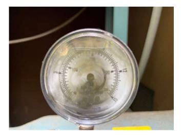
Photo 1: View of the old malfunctioned blower outlet pressure gauge.
