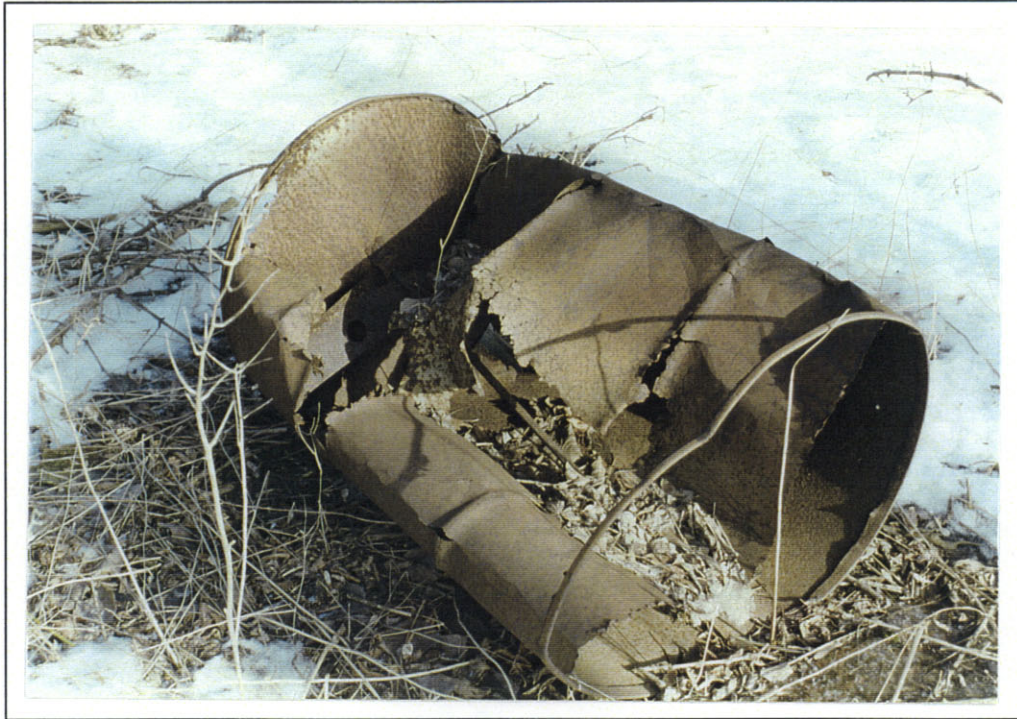
Photograph 5. Heavily rusted and empty drum located to eastern edge of subject site.
