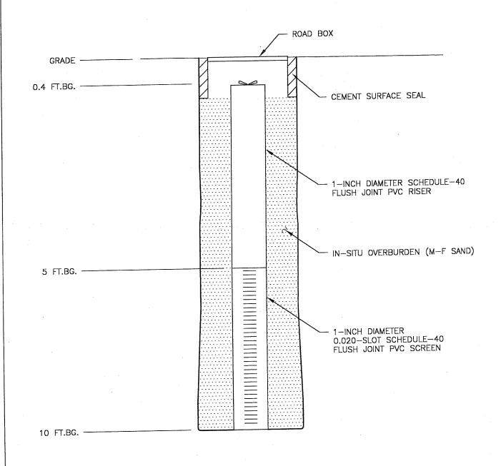
NOTE: TOP OF CASING ELEVATION = 7.96'.
