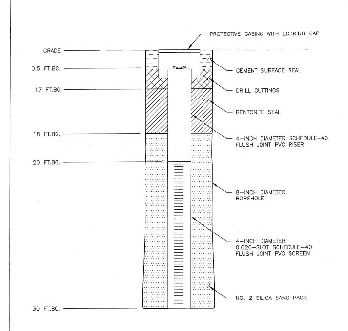
$\frac{\text{NOTE:}}{\text{TOP OF CASING ELEVATION}} = 19.99'.$
