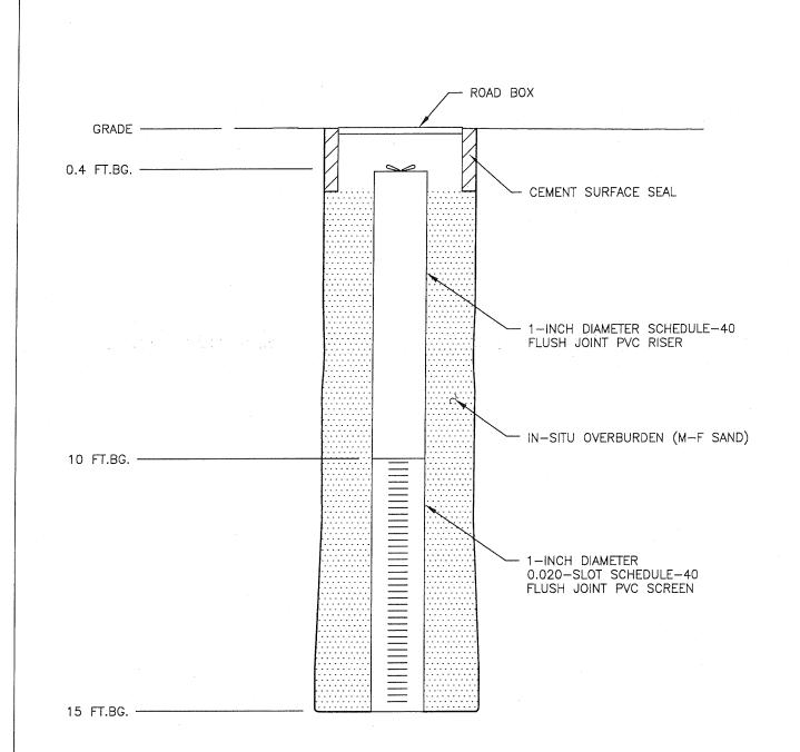
$\frac{\text{NOTE:}}{\text{TOP OF CASING ELEVATION}} = 18.54$ '.
