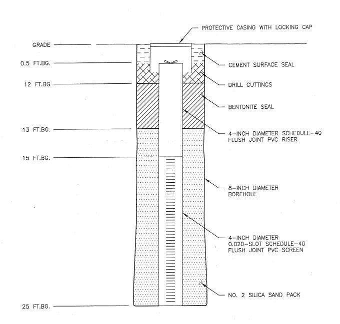
NOTE: TOP OF CASING ELEVATION = 15.14'.
