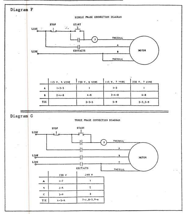
Wiring this explosion-proof blower correctly is essential. Connecting the Pilot Duty Thermal Overload Protection to the proper control circuitry is mandated by UL674 and NEC501. Failure to do so may result in an explosion, and voids EG&G Rotron's warranty. Please contact the Application Engineering Department at the factory if you have any questions.
