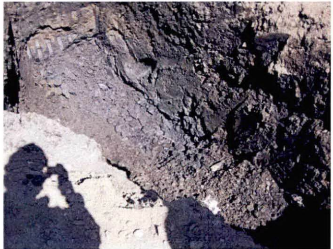
Impacted (stained) soil observed in excavation
