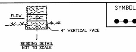
DRAINAGE AREA NO MORE THAN 1/4 ACRE PER 100 FEET OF STRAW BALE DIKE FOR SLOPES LESS THAN 25%.
