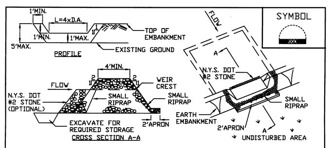
OPTION: A ONE FOOT LAYER OF N.Y.S. DOT #2 STONE MAY BE PLACED ON THE UPSTREAM SIDE OF THE RIPRAP INPLACE OF THE EMBEDDED FILTER CLOTH.
