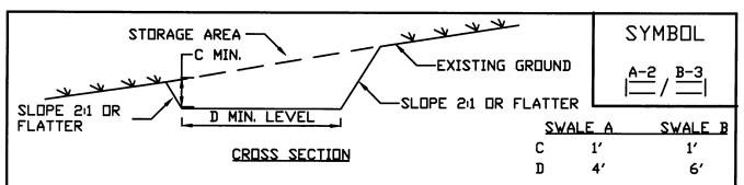
POSITIVE DRAINAGE: 0.5% OR STEEPER DEPENDENT ON TOPOGRAPHY
