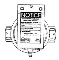
Cut a suitable length of vinyl tubing and attach it to the pressure switch connector on the CHECKPOINT IIa.
