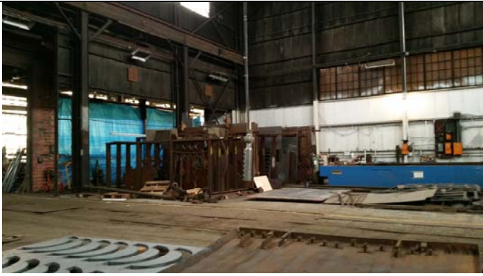
Plasma cutting table in Storage Building & Receiving area of Site Building 2
