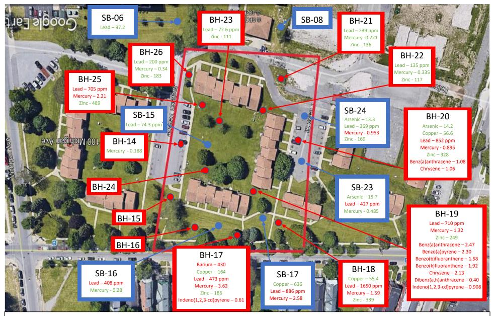
Figure – Boring Locations and Soil Sample Exceedances in ppm
