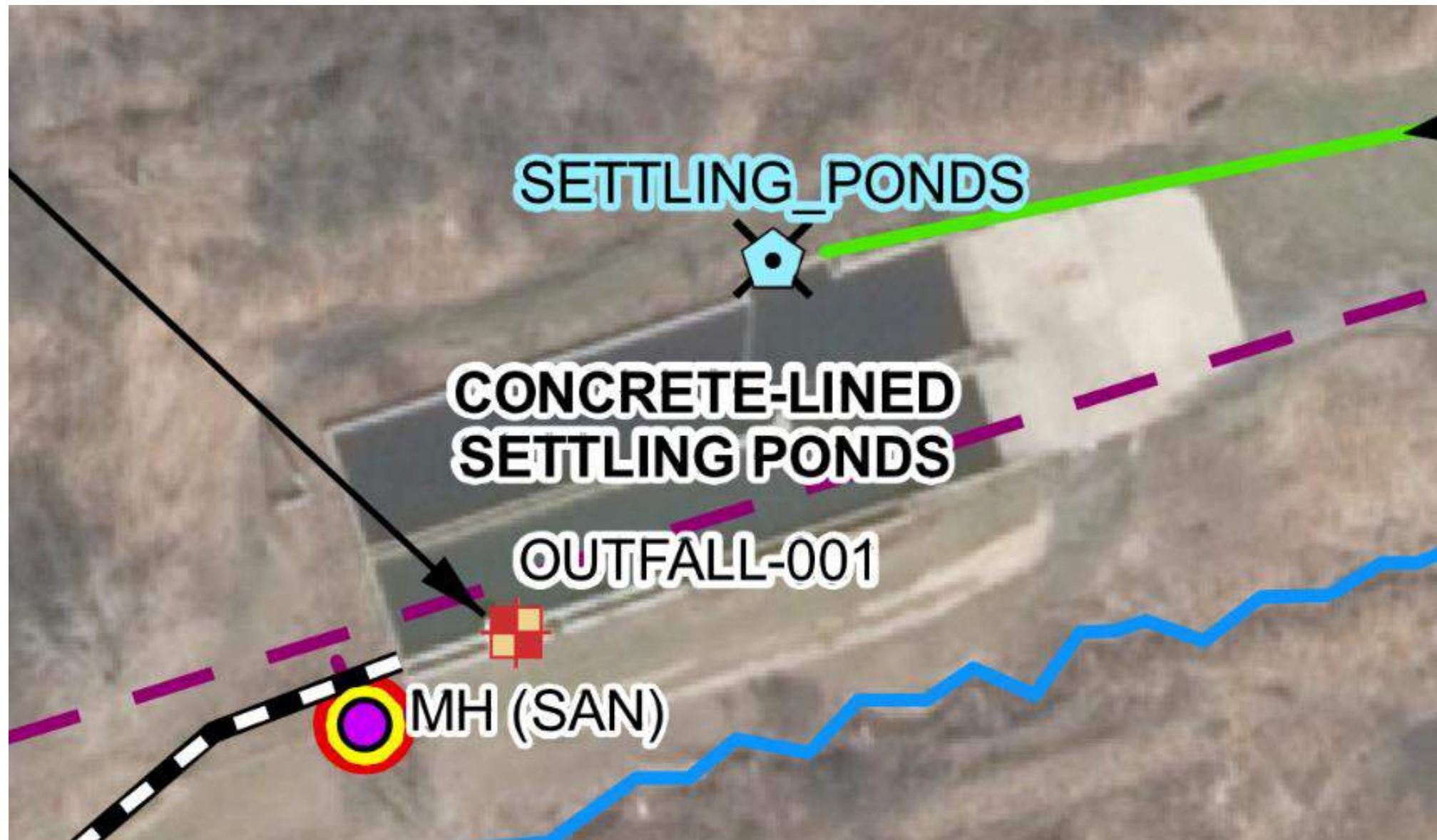
Figure 1a Concrete Lined Settling Ponds Source: O'Brien & Gere (2016)
