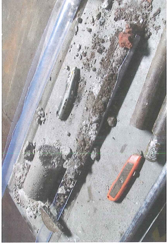
4. Cement core and soil core from 0-4 feet below ground surface at C-1
