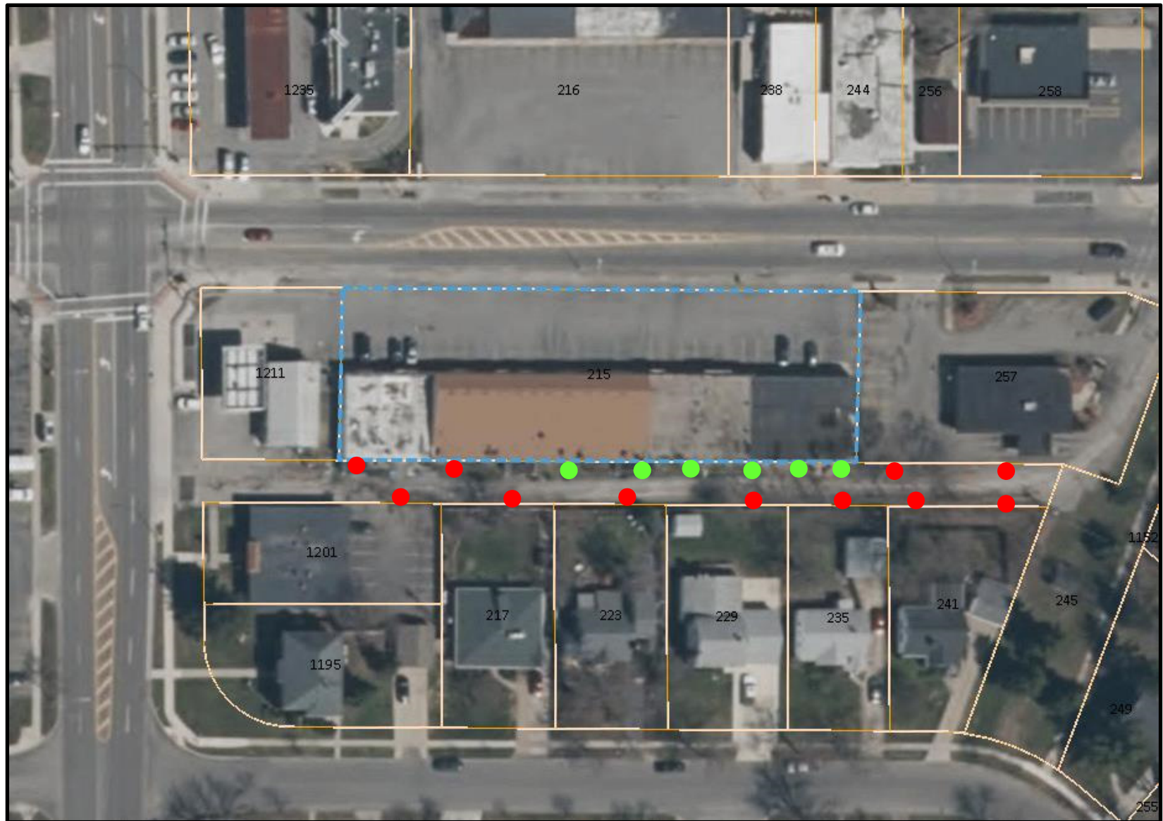
Figure 7. Proposed surface soil sample location map. Green dots are the approximate locations of the samples to be collected from soils placed behind Highland Plaza during construction of the sub-slab depressurization system in the former dry cleaner tenant space.
