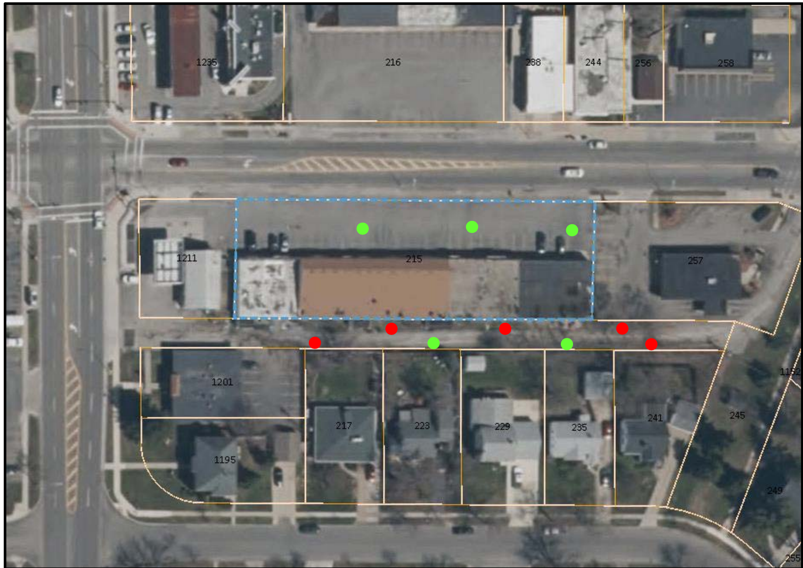
Figure 9. Proposed monitoring well (red dots) location map. Green dots are the approximate locations of the monitoring wells completed during the Remedial Investigation of the Highland Plaza BCP Site.
