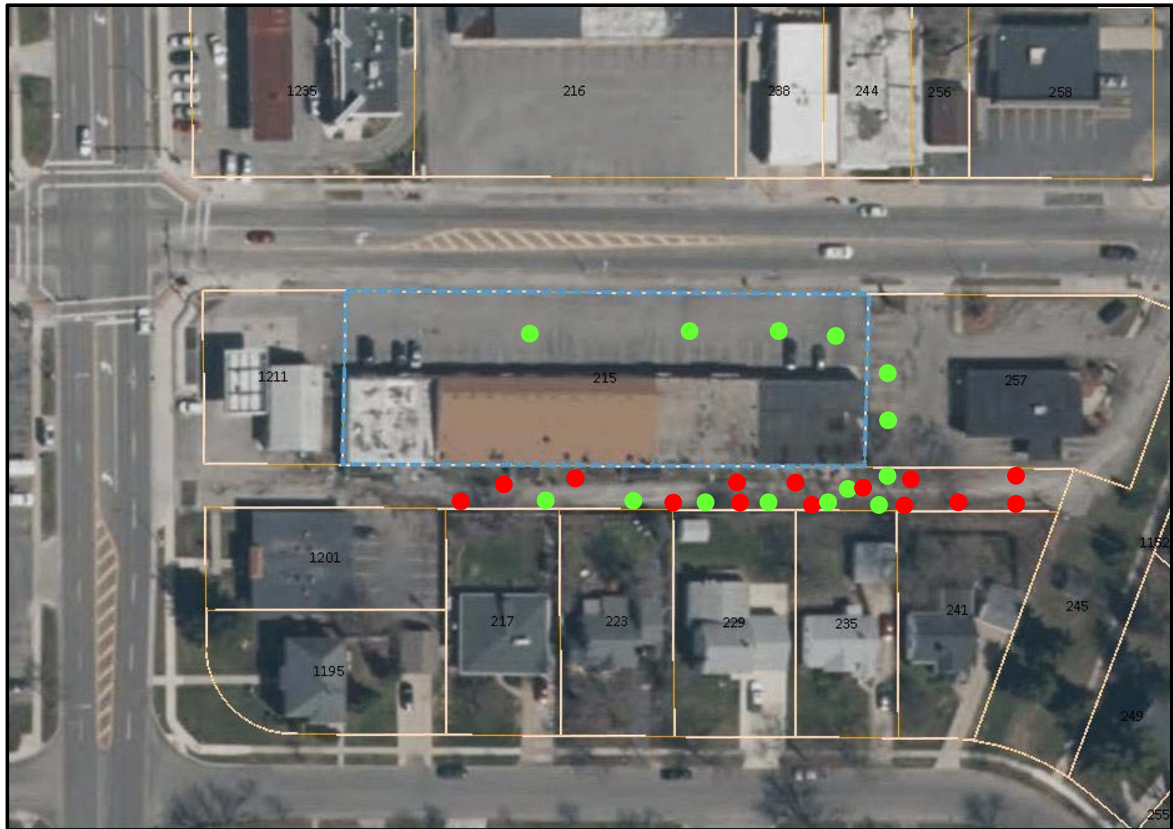
Figure 8. Proposed soil boring (red dots) location map. Green dots are the approximate locations of the soil borings completed during the Remedial Investigation of the Highland Plaza BCP Site.
