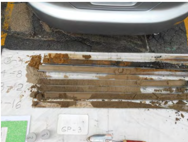
Soil boring GP-3 (4' increments)
