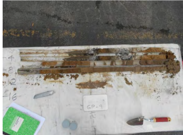
Soil boring GP-9 (4' increments)
