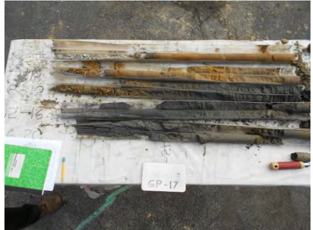
Soil boring GP-17 (4' increments)
