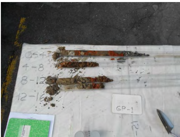
Soil boring GP-1 (4' increments)
