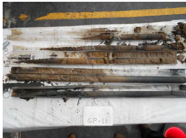
Soil boring GP-11 (4' increments)
