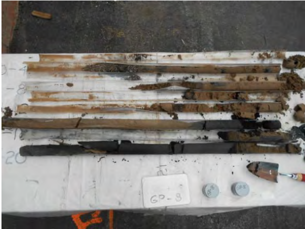
Soil boring GP-8 (4' increments)
