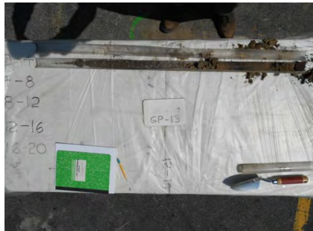
Soil boring GP-13 (4' increments)
