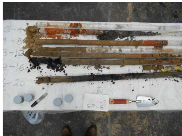
Soil boring GP-6 (4' increments)
