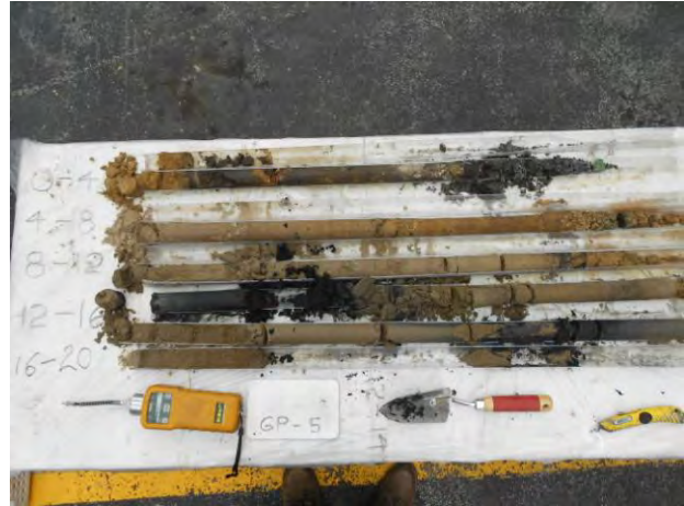
Soil boring GP-5 (4' increments)
