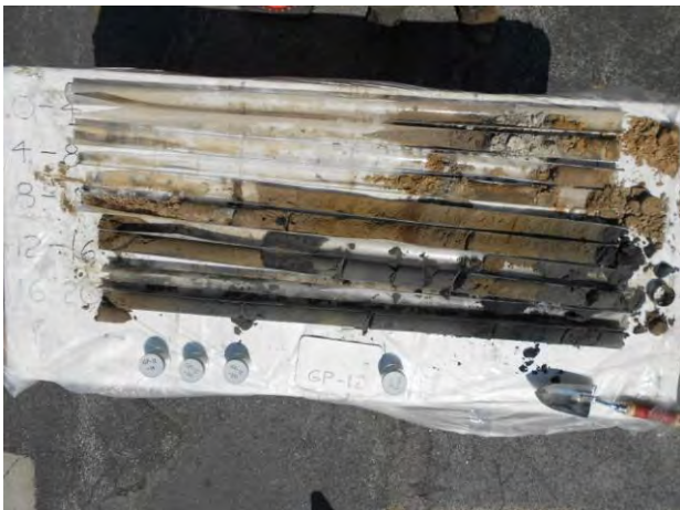
Soil boring GP-12 (4' increments)
