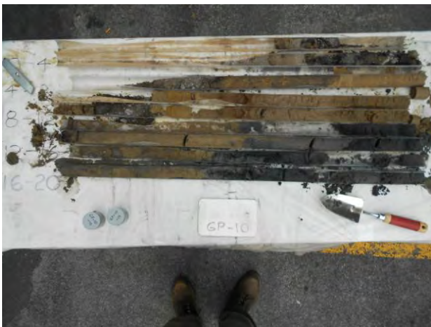
Soil boring GP-10 (4' increments)
