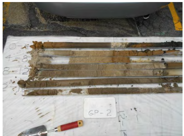
Soil boring GP-2 (4' increments)
