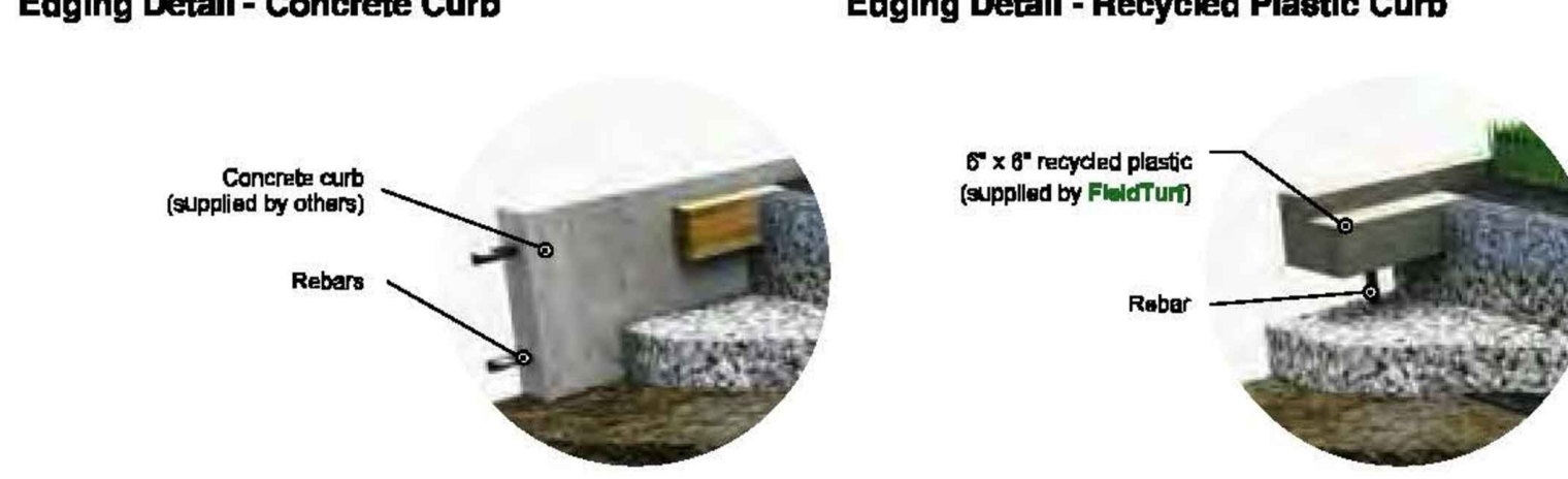
Edging Detail - Recycled Plastic Curb
