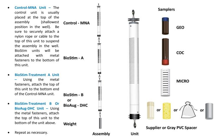
**Figure 1.** Illustration of Bio-Trap Assembly, Unit, and Samplers. Actual configuration may vary depending on the number of samplers and units per well.
