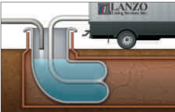
figure1: Direct inversion installation per ASTM F1216
