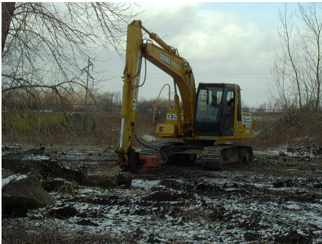
Figure 5 – Deere 102C with concrete breaker attached
