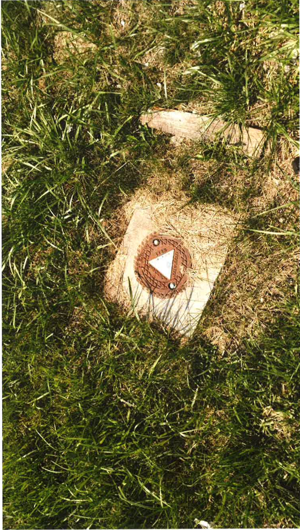
7. A monitoring well.
