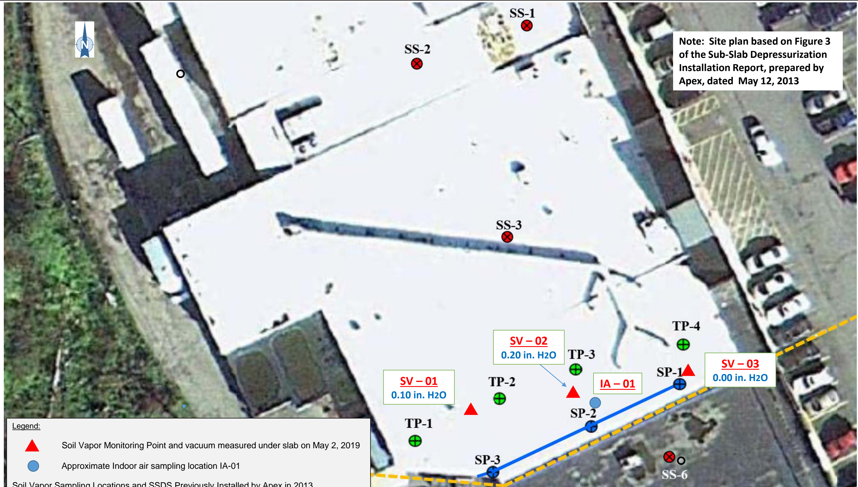
FIGURE 3: Soil Vapor Monitoring Points and Measured Vacuum, May 2, 2019
