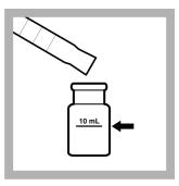
8. **Blank Preparation:** Fill a second sample cell with 10 mL of sample.
