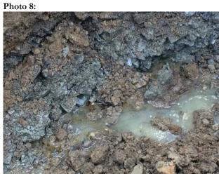
Photo 5: LNAPL and petroleum-impacted soils encountered at TT-3.
