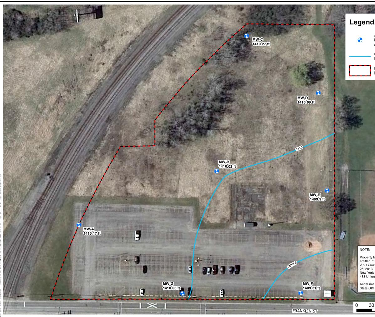
Approximate monitoring well location showing groundwater elevation for November 5, 2014
