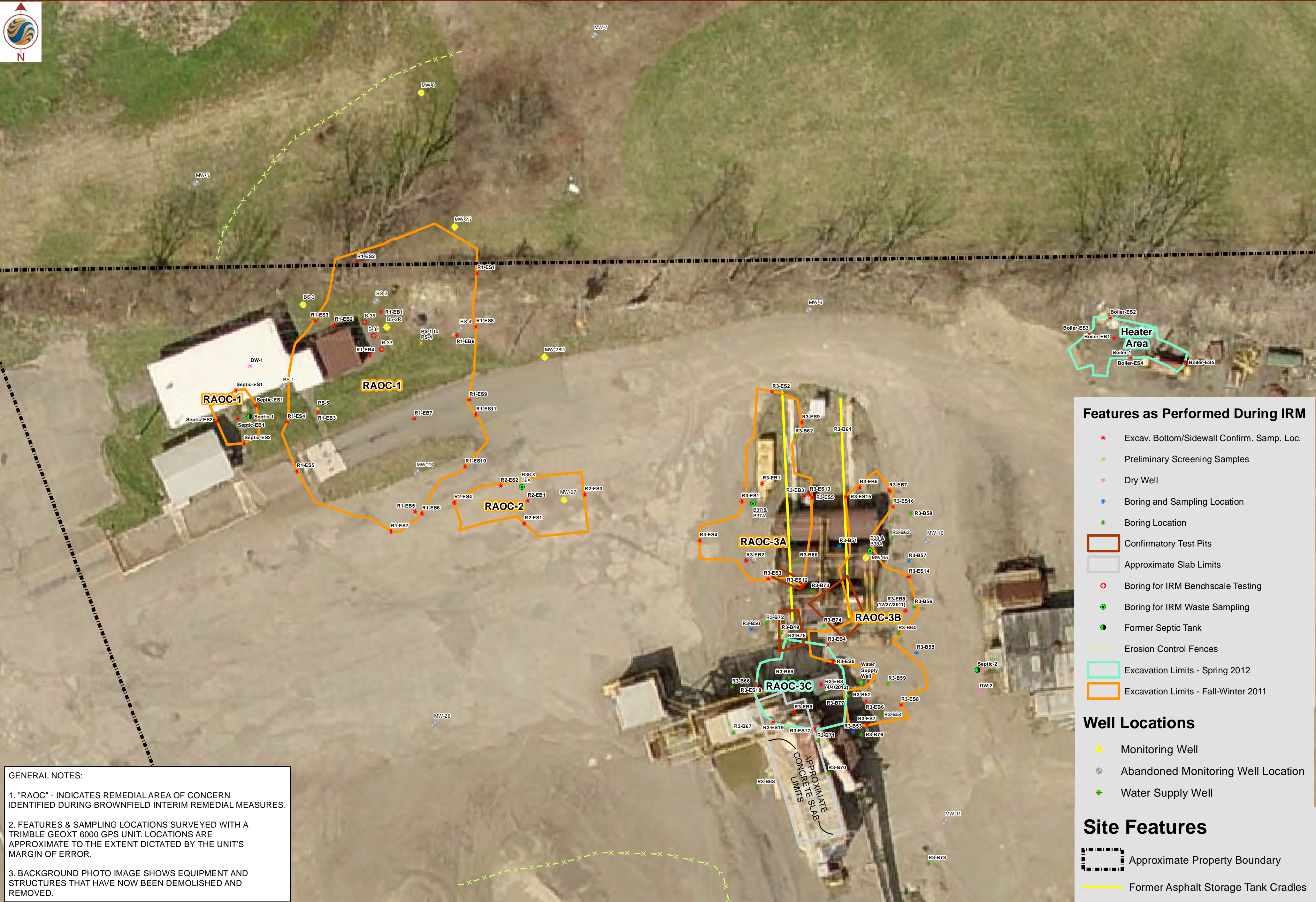
Figure 5: RAOC-1 through RAOC-3 and Heater Area IRM Excavation Limits Alternatives Analysis Report / Remedial Action Work Plan Former Allegany Bitumens Belmont Asphalt Plant Site
