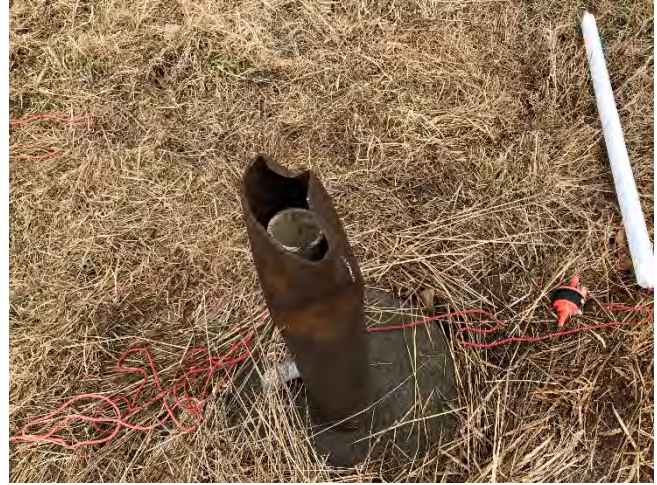
Photo No. 14 OW-1 casing damaged
