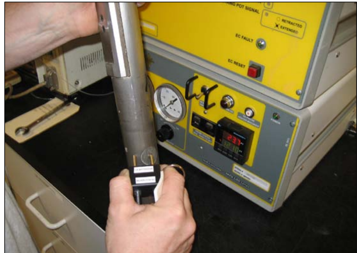
Figure 5.4 Operation of the EC Dipole Test Jig.
