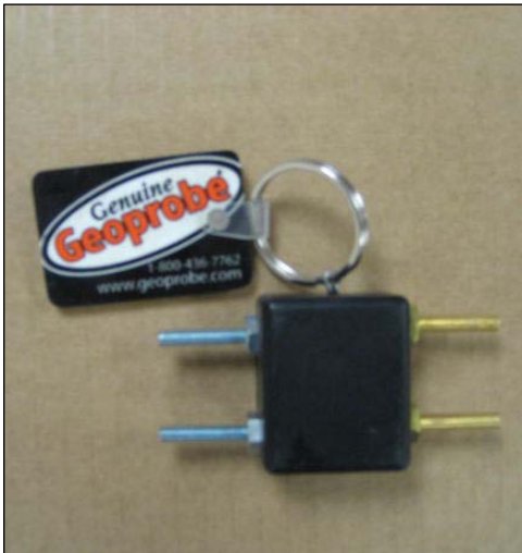
Figure 5.3: EC Dipole Test Jig.
