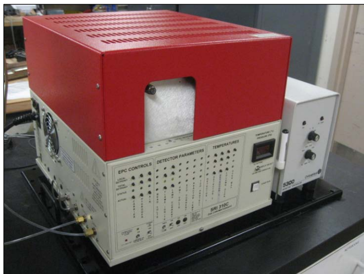
Figure 1: GC1000: SRI 310GC with XSD Controller.
