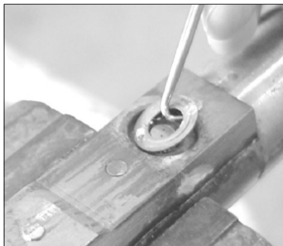
Figure 8.2: Remove and discard the copper washer.
