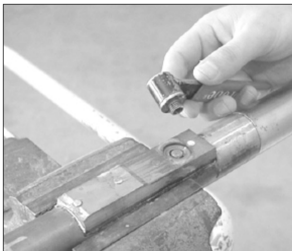
Figure 8.1: Unthread the membrane from the probe block.
