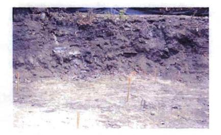
SB-20 sidewall showing brick and debris
