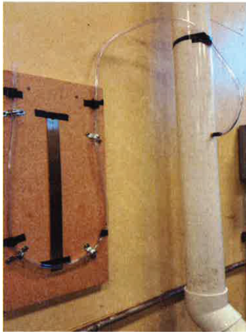
Photograph 13: View of the aqueous manometer installed in the 4-inch diameter PVC EEA duct.
