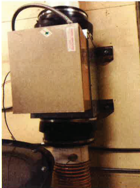
Photograph 14: View of the EM-HX 10 Electric Heater with an 8-inch rubber reducer at both the inlet and outlet. The first G-10P carbon canister is observed in the bottom left of the photograph.
