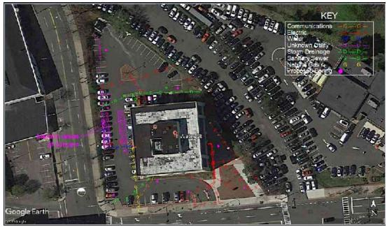
Figure 1. Approximate locations of anomalies, boring locations and utilities delineated on site.
