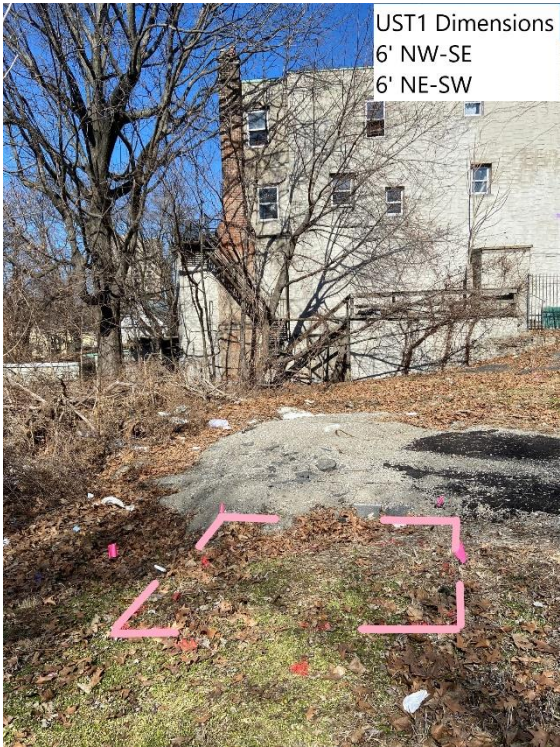
Above is the picture of a possible UST at 2.5' in depth.
