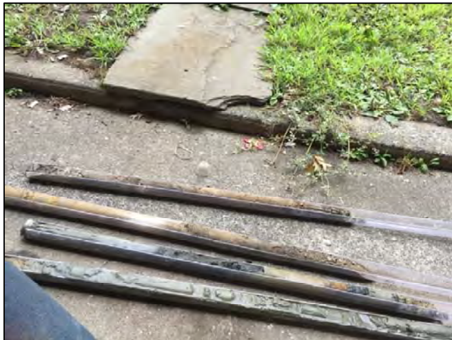
Photograph 3: Soil liners with soil from SB-5.
